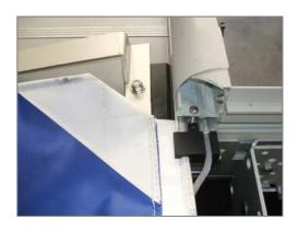
On the motor side of the cover <u>only</u>, we will now insert the magnet that stops the cover in the open position. Remove the tape from the magnet and insert the magnet into the webbing until it is fully inside the webbing. Now slide the glider back against the webbing and into the track.
