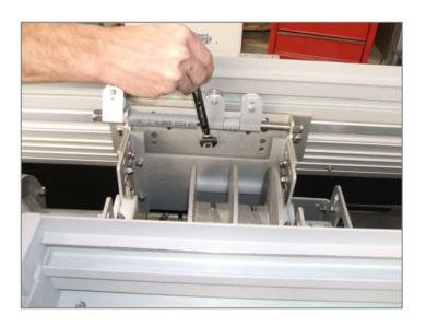
With (1) 3/8" x 1 1/4" bolt, secure the AutoGuard frame to the mounting brackets. There should be (2) bolts total for the motor end, and (2) bolts for the opposite end.
