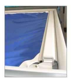
Turn the key to feed the ropes onto the rope reels. BE CAREFUL! WATCH YOUR FINGERS!
