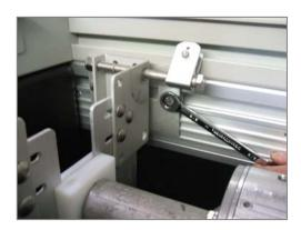
Drop the AutoGuard into the mounting brackets, and align the center mark on the tube with the center of the track. Then tighten all bracket bolts.
